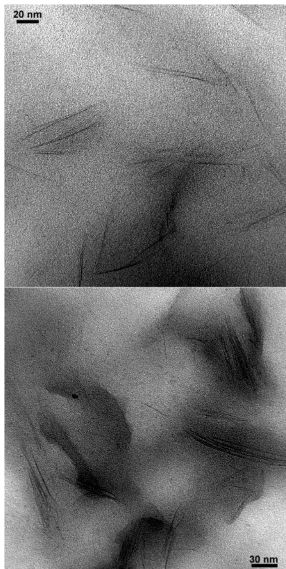
Figure 4. TEM micrographs of the 2.86 vol % Nanofil 804-PU composite.
